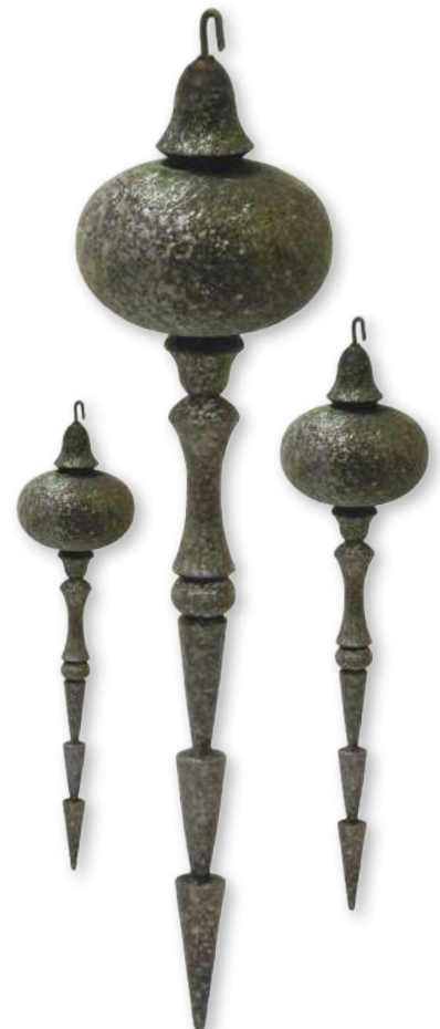
▲ Pic.6 The bulbous bit at the top of the icicle is a simple bead. The pencil line in the centre is a guide for me to turn the bead evenly – the spindle gouge is perfect for this, but use the skew if you are confident in doing so
